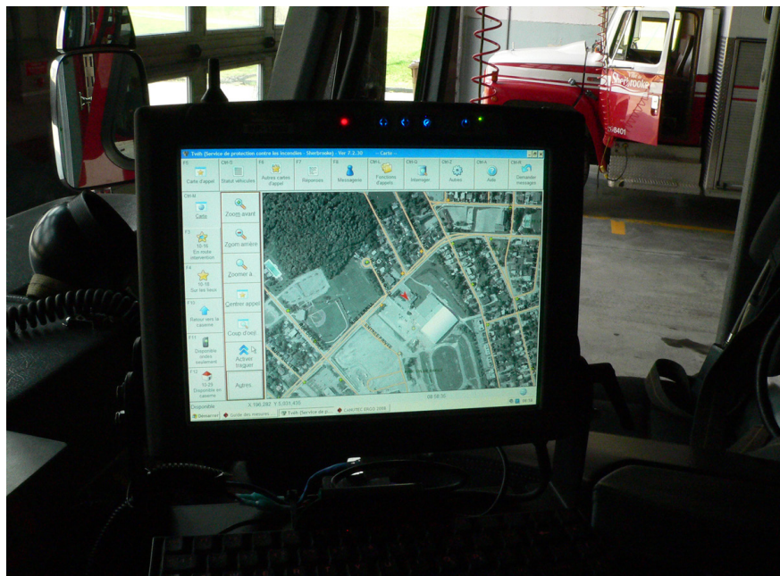
At right: MrSID imagery being used in a Versaterm dispatch application in the cab of a fire truck in the Sherbrooke fleet. Updated imagery is pulled to the Datalux Tracer terminal in each vehicle over a wireless network
