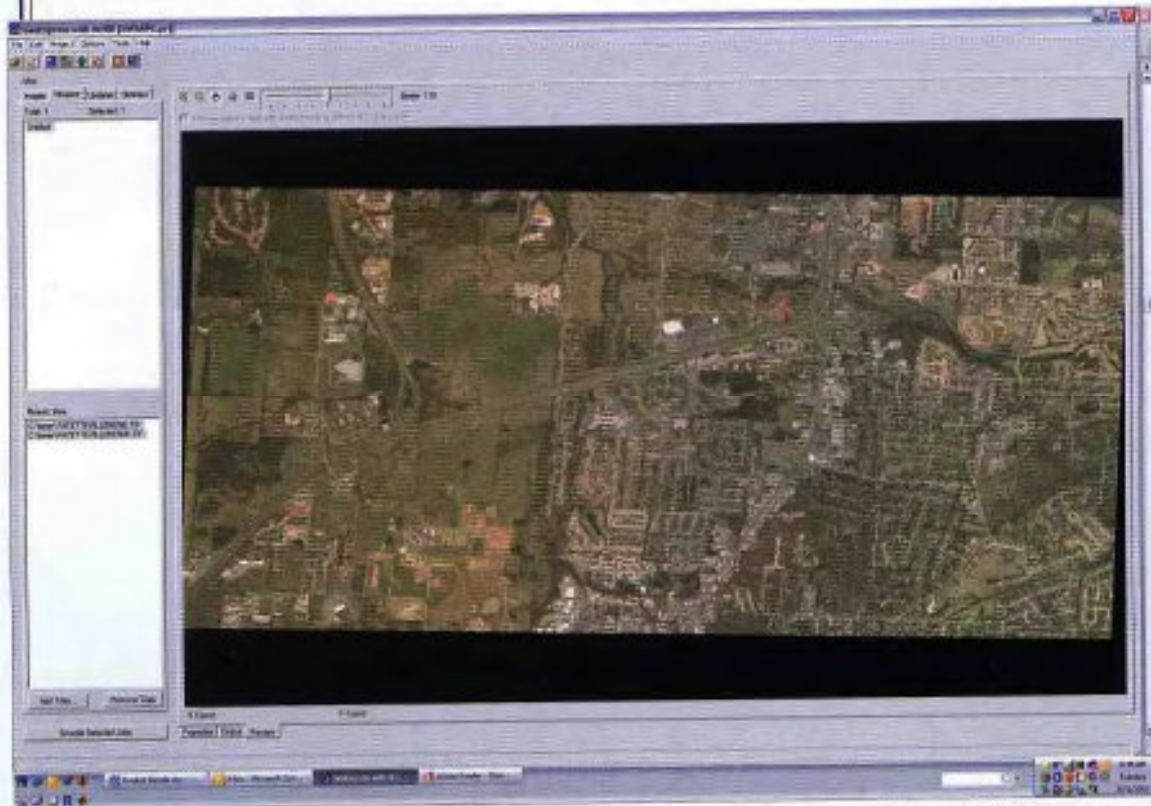
Two 350MB GeoTiff files in the State Plane system were reprojected and mosaicked in geodetic coordinates on WGS84.
